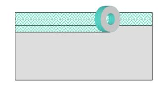
2 Lay out patch film on flat surface. Affix transfer tape to patch (side by side) until entire patch is covered. Ensure all air bubbles are rolled out.
