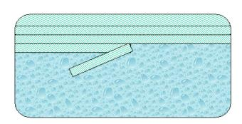
3 Cut patch a minimum of 100mm larger than the damaged area. For larger patches allow at least 200mm extra. Radius corners. Remove strips of backing paper to reveal adhesive.
