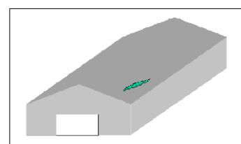
1 Ensure the greenhouse film and patch film surfaces are washed clean, dried and patch installed in ambient air temperatures above 10°C (50°F).
