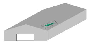
Place patch over damaged area of film. Press/roll out air bubbles to provide full adhesion. Wash hands after use. Note: In some instances an inside patch may be required to support the outside patch.
