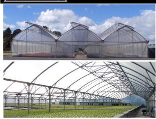
Top of the line greenhouse models from Redpath. They are fully NZ building code compliant design engineered structures, utilising strong RHS steel, HDG poles, 12mm fully bolted 4mm plate connections, and cold rolled 'walk-through' wide steel gutters as standard.
